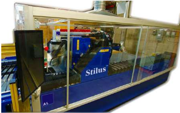
The Advanced Lasers, Inc. Stilus® cutting machine features the Iradion 1625 Laser, linear drives and patented CAD/CAM software.
