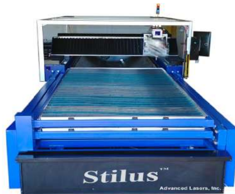
The Stilus® has dual pallet cutting tables to maximize part production.
