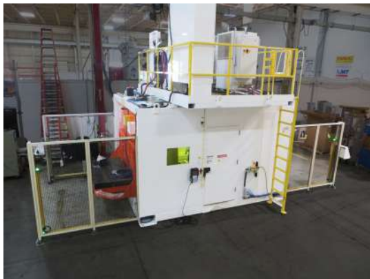
DRS dual turntable system enhances productivity by facilitating part loading during the cutting process.
