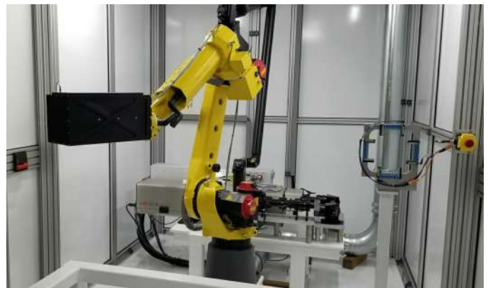
The DRS Application Lab features a robotic cell with the OEM65ix 650 watt laser. Note the scanner head.
